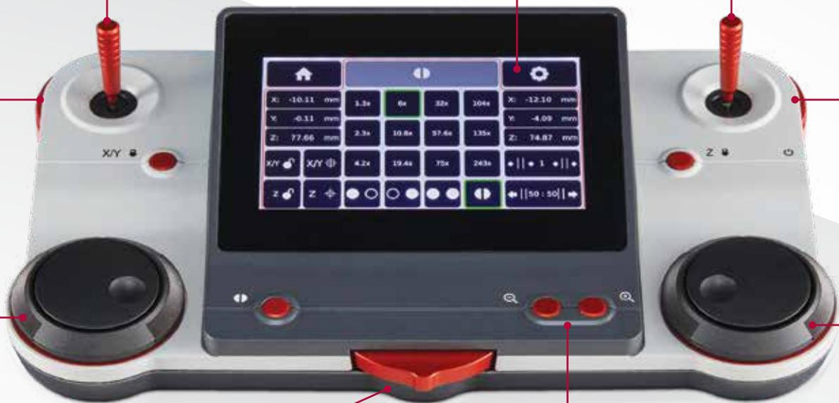
Viewing options for Full Left, Full Right, Transparent Overlay and Adjustable Split with smooth scrolling dividing line for sliding across parallel regions of interest
